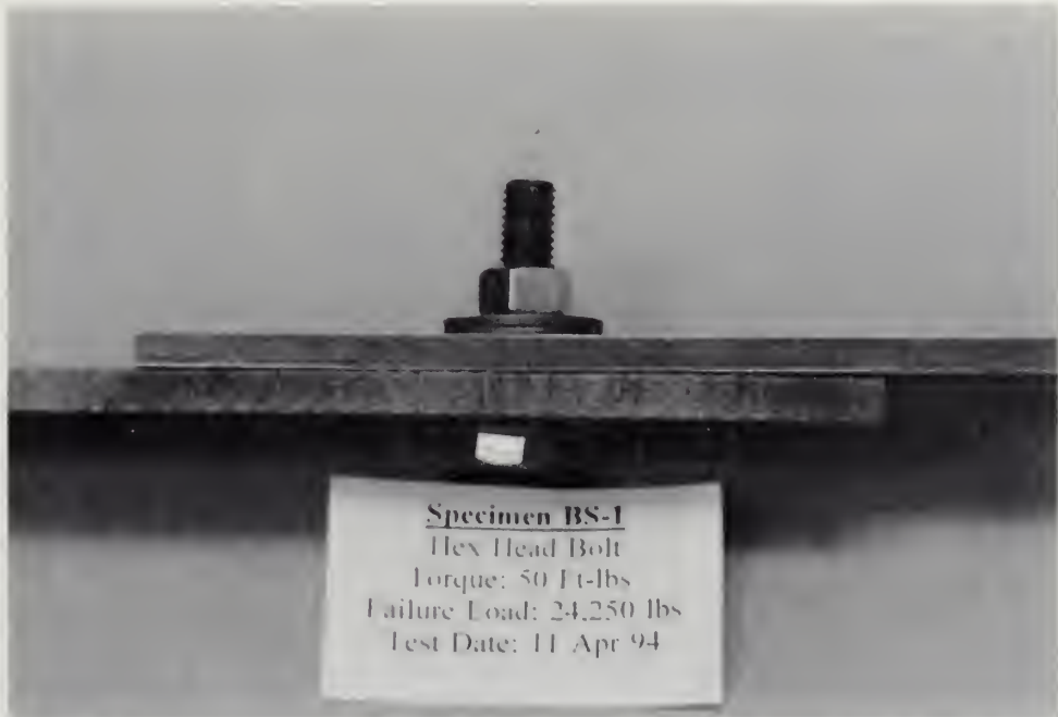
Specimen BS-1, Hex Head Bolt, 50 ft-lbs torque. Edge view of joint showing bolt bending and washer dishing.
